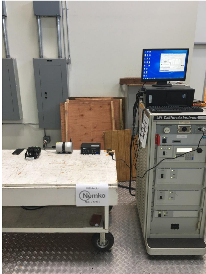
Figure 8.11-1: Voltage dips and interruptions setup photo
