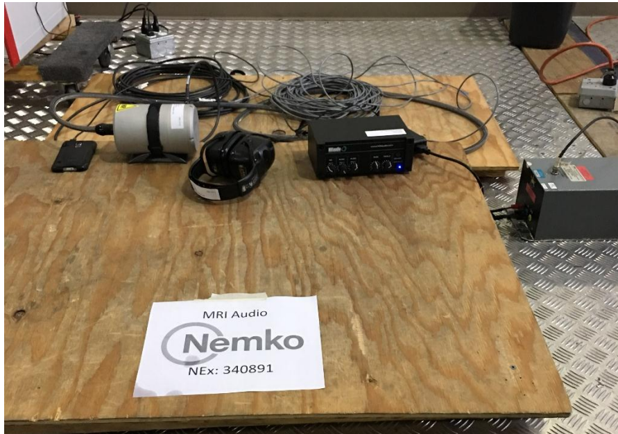
Figure 8.7-1: Conducted disturbances induced by RF fields setup photo
