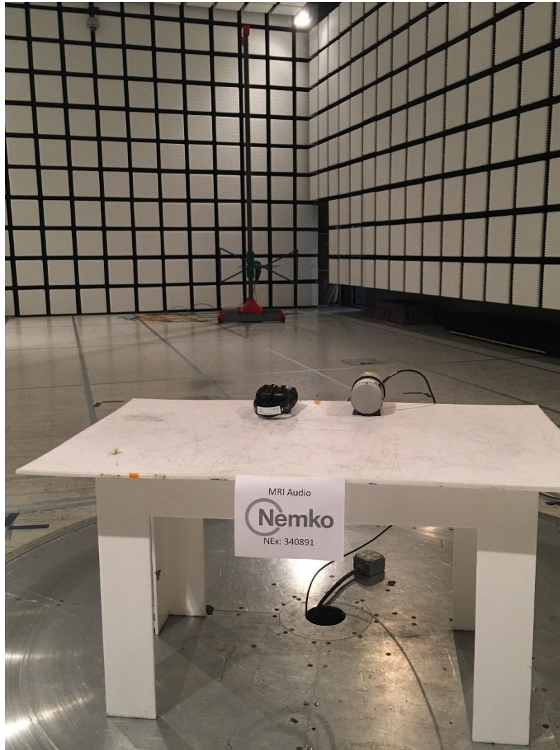
Figure 8.1-2: Radiated RF emissions setup photo
