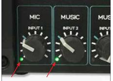
**8. MIC AND AUDIO CONTROL KNOBS** The knob **MIC INPUT 1** controls the technologist microphone to the patient. The knob **MUSIC INPUT 2** controls the patient's headphone volume. Both knobs have a green indicator light when in use.
